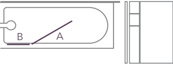
A: Moving Panels (screen width when folded into the bath 712mm) B: Fixed Panel Recommended shower head position
